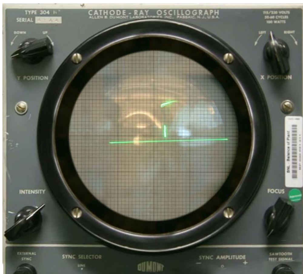
Figure 2: Tennis for Two on a DuMont Lab Oscilloscope Type 304-A
