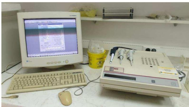
**Figure 8.** Microtox model 500 Analyser (Azur Environmental, Carlsbad, USA) used for the toxicity assessment of sea water, sediment and mussel biological tissue samples.
