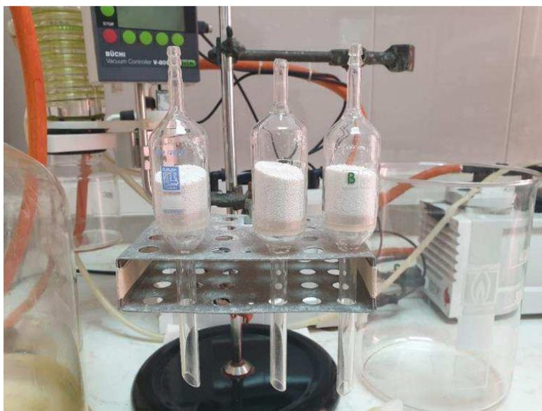
**Figure 5.** Amberlite XAD-7 resin columns (20 ml) used to concentrate all nonpolar compounds from the seawater.
