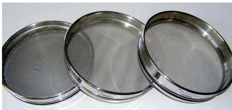
**Figure 4.** Sieves used to separate fine-grained from the coarse-grained sediment fraction.
