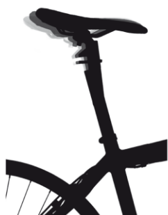
Figure 3. An adjustable saddle position, which enables the cyclists to adjust the angle and position of the saddle by putting it into three different positions: (1) horizontal position (normal), (2) 10% angle of the saddle and (3) 20% angle of the saddle. Note that the forward movement of the saddle and optimized saddle angle does not alter the saddle height.
