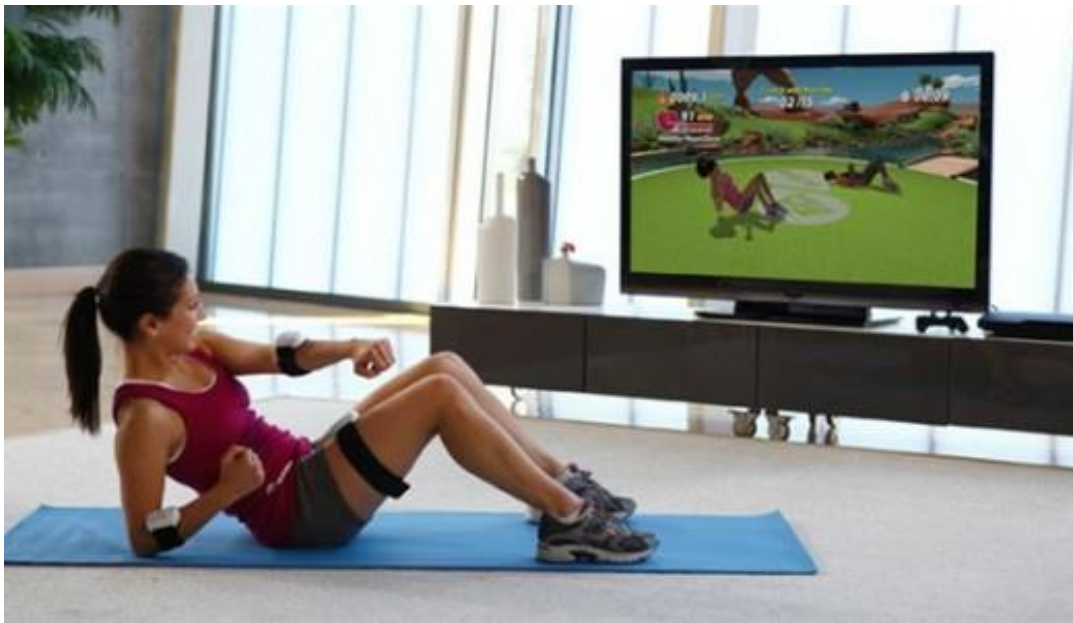
Figure 7: Kinect motion sensor can easily track a position and pose of human body, this way it can be a great zumba trainer keeping track on correctly executed moves.
