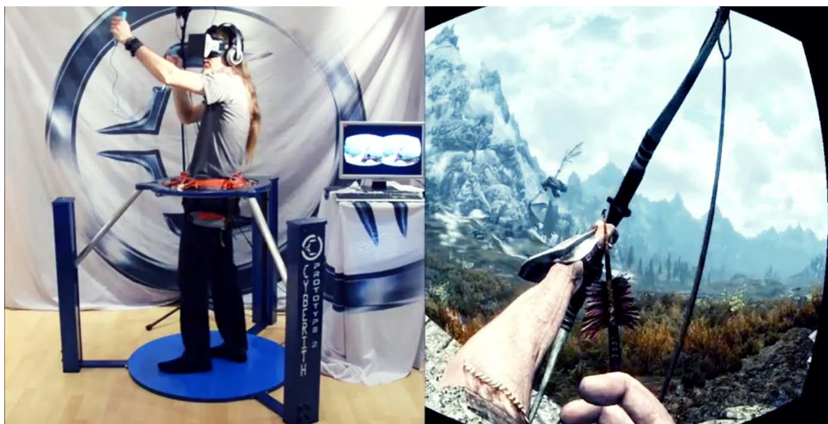
Figure 8: Cyberith Virtualizer combines VR headsets, with player movement recognition and detection of vertical movement forces to create an virtual experience where full body presence is required to interact with game world.
