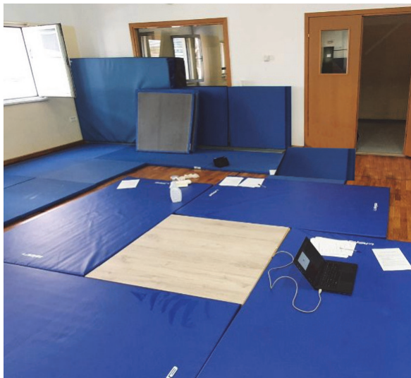
Figure 1 The picture was taken during the data collection event, where fall events were simulated following safety precautions. The smart floor is the white surface surrounded by landing mats.
