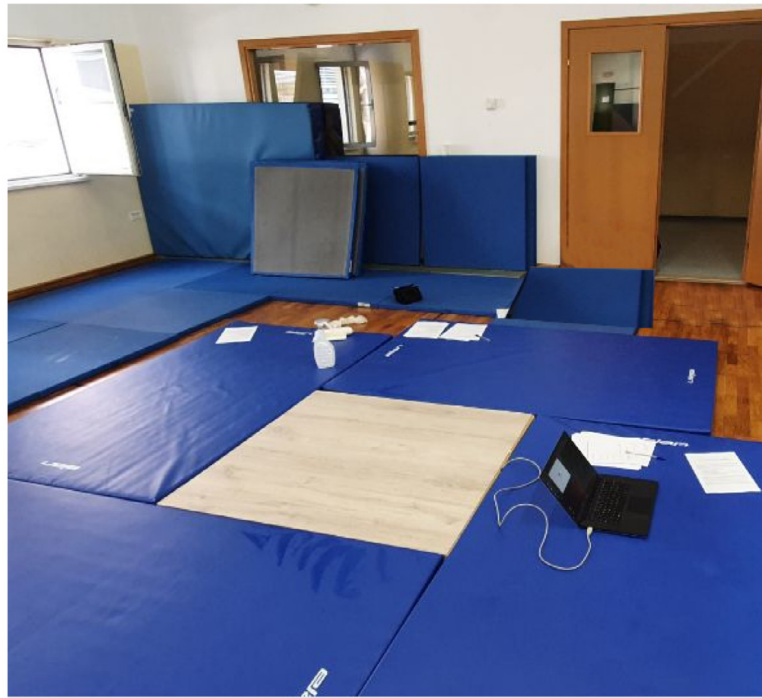
Fig. 4. Data collection set-up: The smart floor is the white square surface surrounded by landing mats. It differs from Fig. 3, because covered with the laminate layer. Notice the laptop linked to the smart floor for data acquisition.
