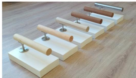
Figure 1. Handrail samples (from left to right: unmodified spruce, unmodified pine, acetylated radiata pine, thermally modified pine, stainless steel).
